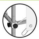
2 ATTACH VINYL PANELS USING ELASTIC O-RINGS
