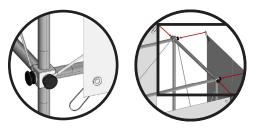
2 ATTACH VINYL PANELS USING ELASTIC O-RINGS
